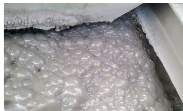
Figure 27—Froth with reduced depressant dosage and air rate adjustment
