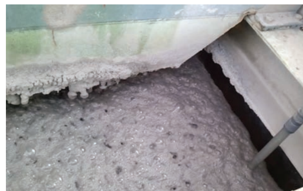
Figure 26—Froth with excessive depressant dosage
